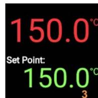
The "3" light on the controller display indicates that the valve is set to open.
