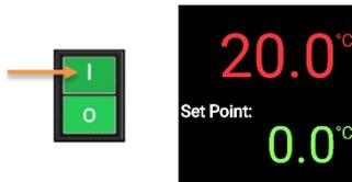
Place the oven **Power Switch** in the ON ( I ) position.
