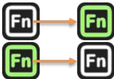
Pressing the **left FN** button activates heating Program 1, turning the button green to indicate it is in use. Pressing the button again during operation will terminate Program 1.
