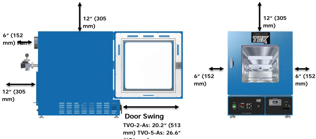
**6 inches (152 mm)** of clearance is required on the sides.
