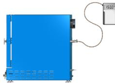
3. The oven chamber must be **empty, sealed** and be **under vacuum**. See the [Evacuating and Backfilling the Oven Chamber](#) topic on page 46.
