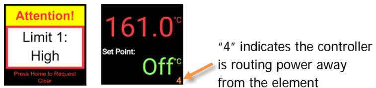
Alternating alert screens flash when the high limit heating cutoff is active.
