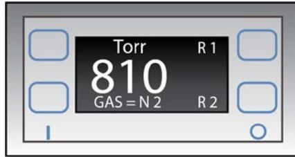
Shows the chamber pressure level in torr and millitorr (mTorr). The gauge that this display connects to measures the pressure of pure nitrogen (N<sub>2</sub>) and is used to control the automated backfill function. Backfilling is commonly done using N<sub>2</sub> or other inert gases.
