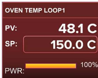
**PV:** The present oven chamber temperature. When the chamber is pumped down, this **Process Value** measures the temperature of the shelving in the vacuum environment. When atmosphere is present in the chamber, the PV is a measurement of that gas temperature.
