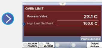
Use the [Set the Oven Limit Temperature](#) procedure on page 44 to set the Limit heating cutoff at least 10°C above the highest intended temperature of your application.
