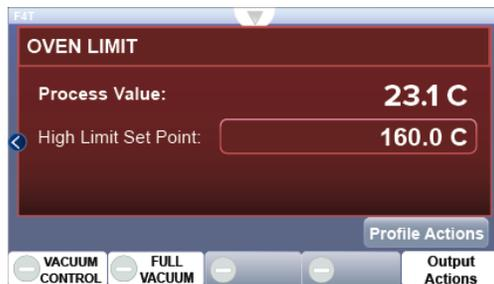
The Oven Limit system routes power away from the heating elements during over temperature events, preventing further overheating. See page 41.
