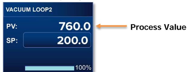
2. **Record the chamber pressure** level showing on the Vacuum Gauge display.
