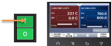
Place the oven **Power Switch** in the ON ( I ) position.
