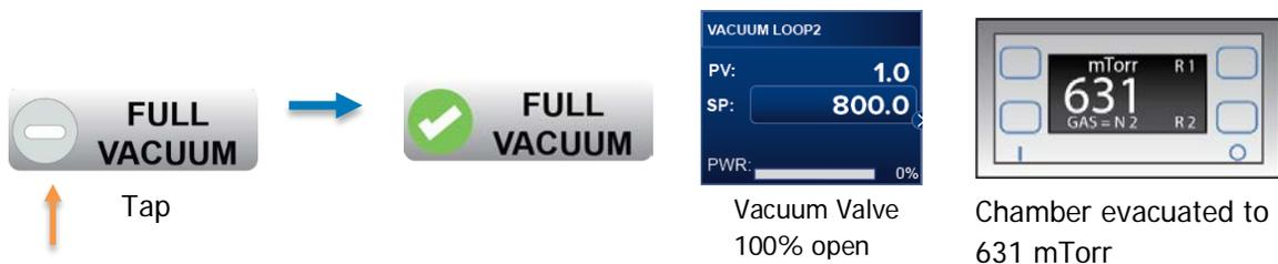
**Reminder:** The homepage vacuum tab cannot display a Process Value of less than 1 torr.
